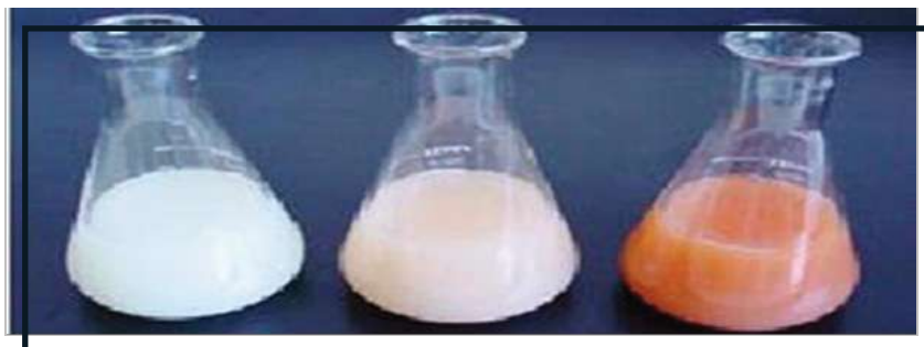
Fig 2: Colour change at the end point from white precipitate at the beginning of the titration to reddish brown precipitate formation.
